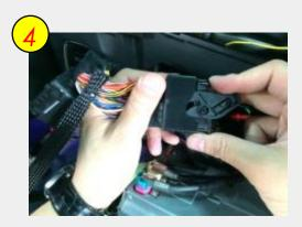
Connect the bunch of original cables to the provided power cable (Femsletions.comptor)
