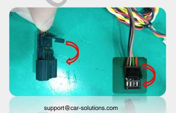
\* Please find locker on male and female connector of supplied I-Drive power cable, once open the locker you could easily change the pin arrangement and lock it.
