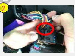
Connect the optical fiber cable to the supplied power cable
